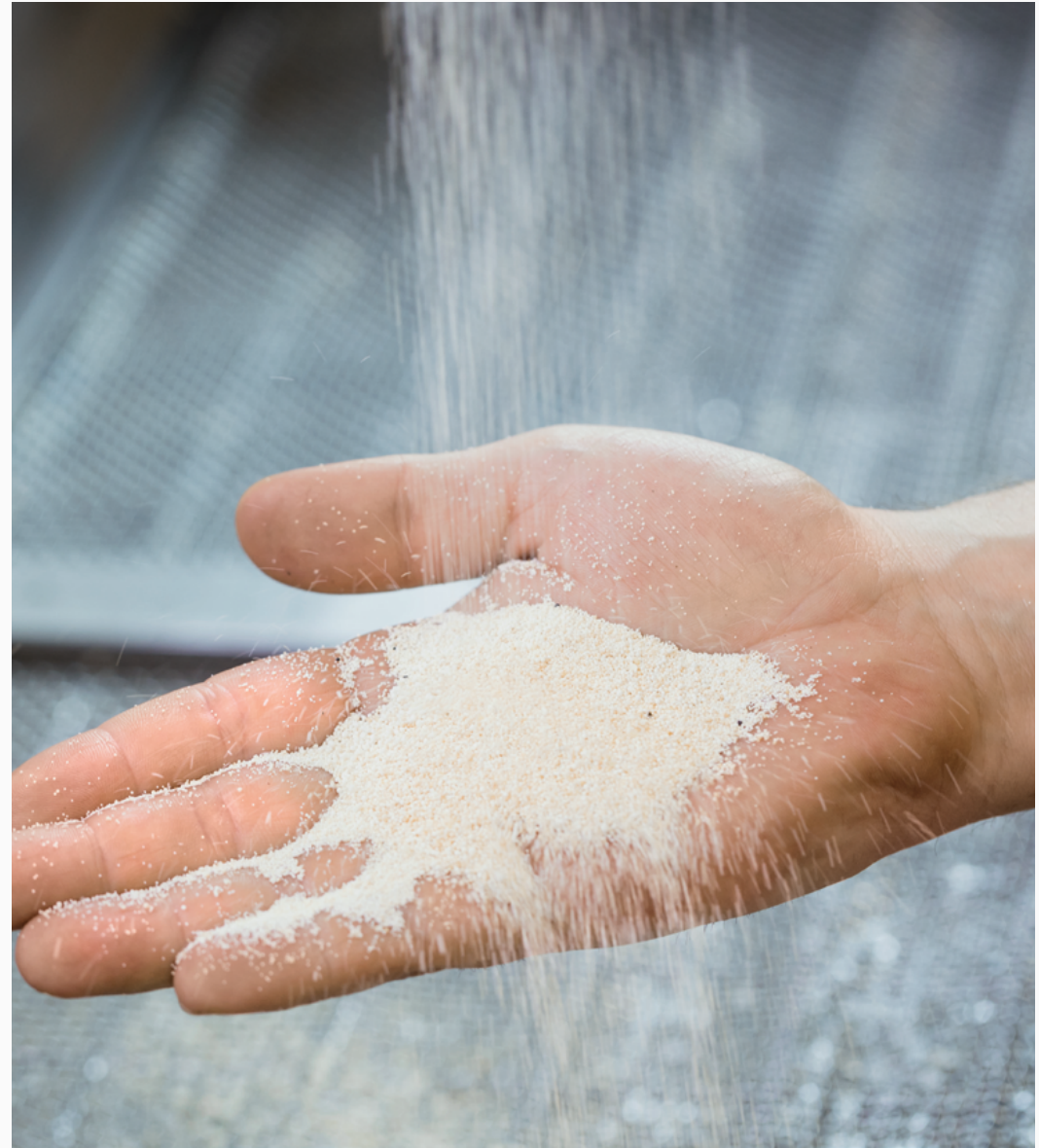
At the end of the recycling process, the filter material has the same quality as new material. By using it in new cartridges we close the material cycle and save valuable resources.
