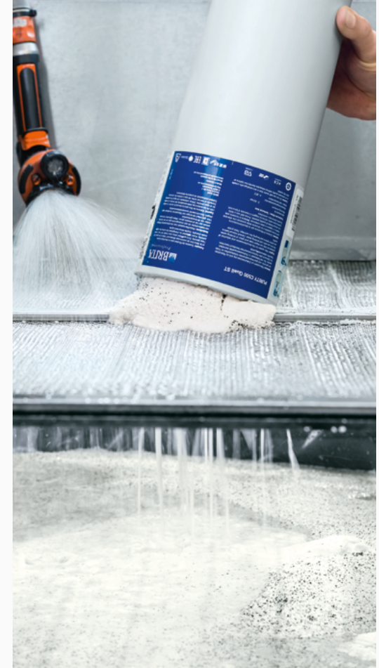
The returned cartridges are opened and emptied manually and the filter material is prepared for the regeneration process.
